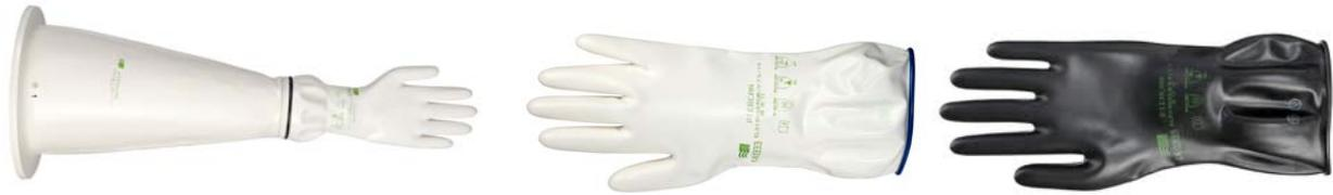
Like the one-piece dipped gloves, Accordion and Straight sleeves can be attached to drybox/isolator box ports. For some manufacturing or R&D environments, the total lifetime cost of ownership will be lower for a sleeve-and-glove combination rather than a one-piece glove system because when one-piece dipped gloves wear out in any part of the entire glove, the whole pair must be replaced.
