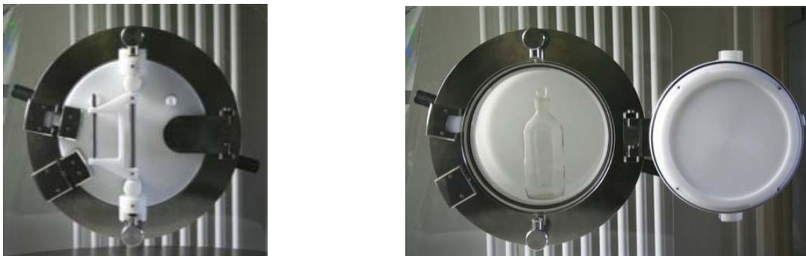
The Rapid Transfer port consists of the Passive (Beta) canister or bag attachment and the Active (Alpha) port which is connected to a sealed / controlled enclosure such as an Isolator or glovebox.
