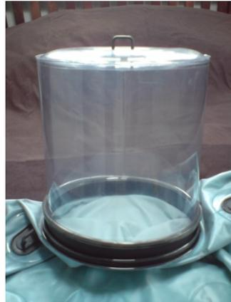
Unlike full air suits, half-suits can be operated comfortably for quite extended periods of work and may be used either standing or seated. The operators can leave the suit at any time for breaks, without compromising the isolator environment. Entering and leaving the suits takes a little practice, but is very much quicker than the gowning process required for conventional cleanrooms.
